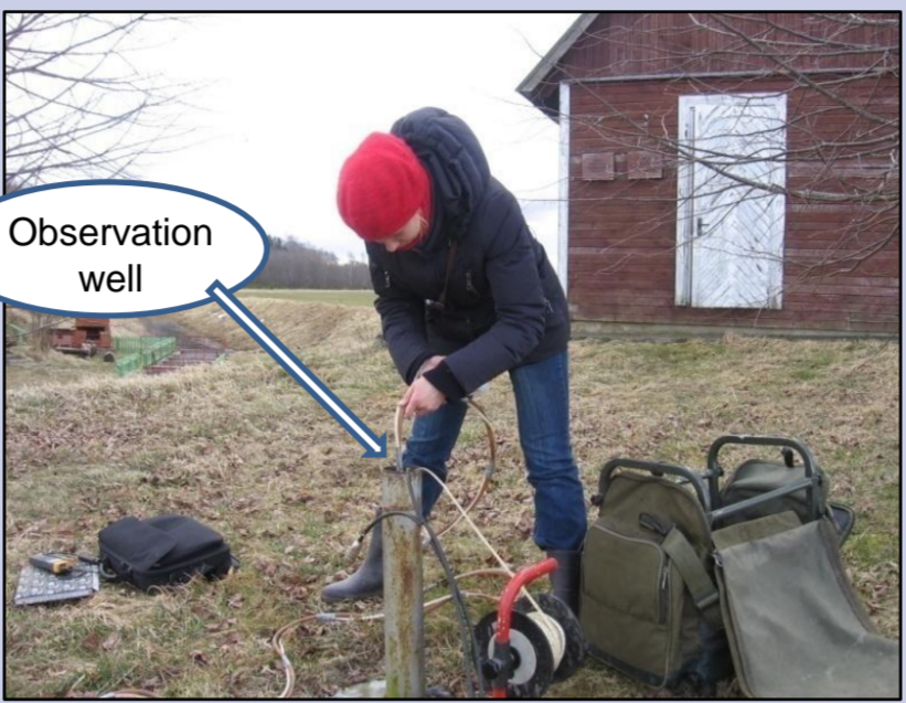
Figure 2. Collection of groundwater level data
