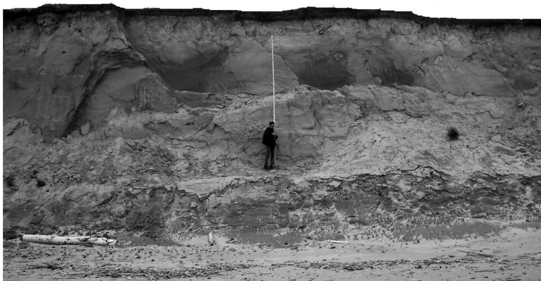
Figure 3.23. The sand rich overconsolidate diamicton interpreted as local deformation till at the Strante site. The stick at the hands of author is 5.0 m long. The location of the image is approximately at the 30,700 m profile mark indicated in the figure 3.25.
